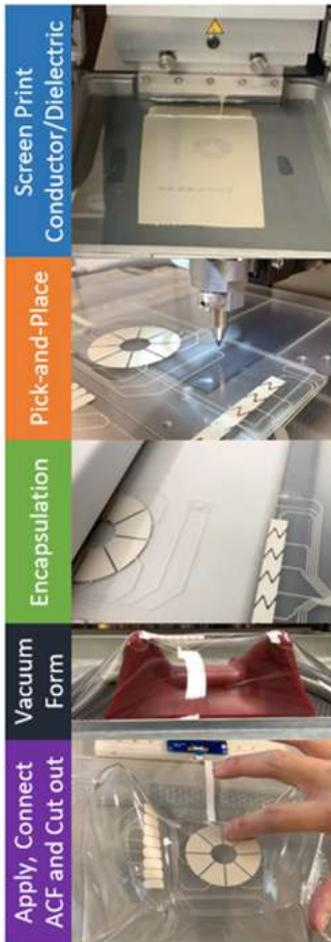
**Figure 1:** Proposed In-mold Electronics fabrication process.
