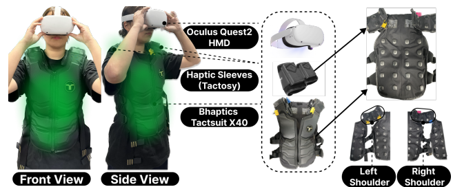
Figure 4: Overall hardware configuration. Users wear a customized haptic vest along with haptic sleeves on both shoulders.
