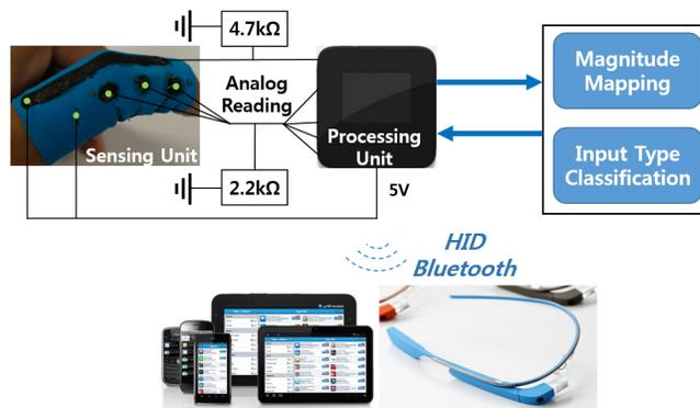
Figure 3: TIMMi schematic workflow
