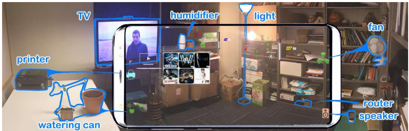
Figure 1. Scenariot is a method for discovering and localizing IoT devices with a SLAM-based AR device. We register the discovered devices spatially in the AR scene to enable new spatial aware interactions.
