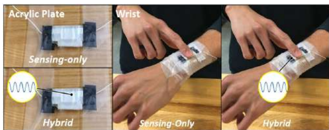
Figure 11: Study setup to measure SNR for two operation modes ( Sensing-only & Hybrid ) on different mounting surfaces ( Acrylic Plate & Wrist ).
