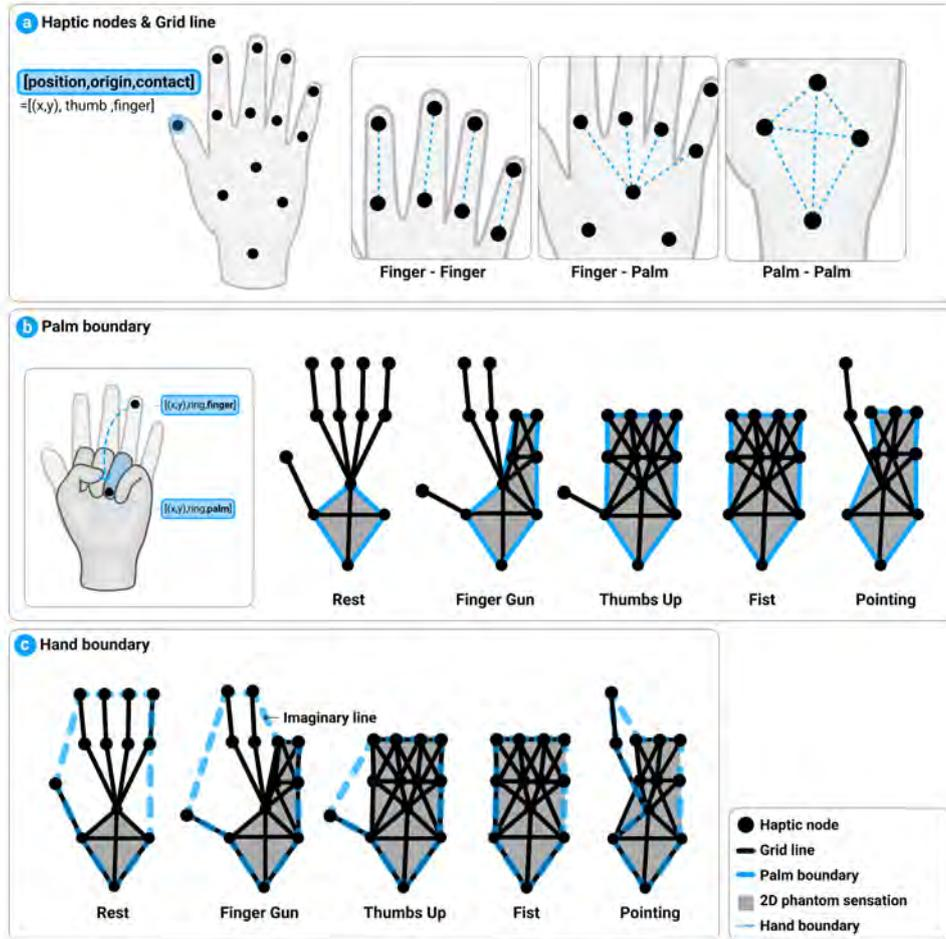
Figure 3.5: (a) A haptic node contains  $(x,y)$  position, origin, and contact. Connecting adjacent haptic nodes on the finger and the palm form grid lines. (b) We form palm boundary utilizing the haptic nodes on the palm which expands if the finger is folded for different hand postures. (c) The hand boundary is set to encompass the outermost grid lines and extra imaginary lines are used to complete the closed hull.
