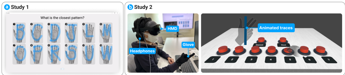
Figure 4.1: The setup overview of studies for (a) 1D & 2D phantom sensation recognition for whole-hand and (b) similarity for posture-adaptive haptic rendering evaluations.
