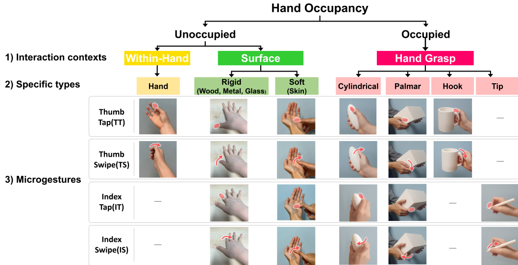
Figure 2: VibAware supports a set of gestures categorized in Within-hand , Surface and Hand Grasp . Each context has a more specific type with a tap and swipe gesture.
